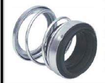
The seal can be use regardless of direction of rotation since the driving torque is not transmitted through the coll spring. The required driving torque is enhanced through the unique rubber bellow which fits on the shaft through the interference fit between the collar, rubber bellow & the shaft.
