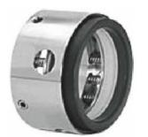
These Seals can be easily assemble or dismantled through circlip provided & cab be change to Balance version of its type merely by changing the carbon face only & an be provided with single, double or tandem arrangement worth external seal support systems & devices.
